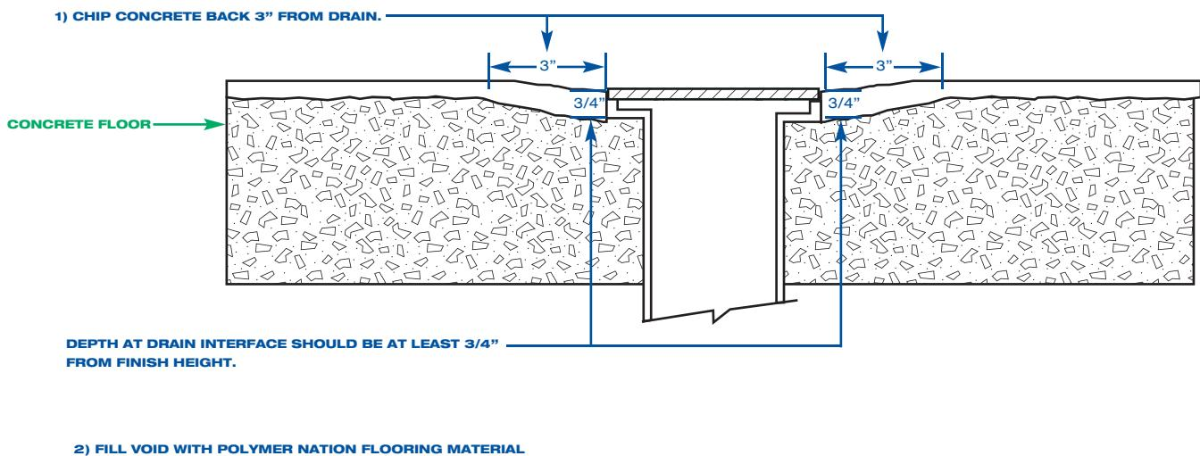
IF A LIGHT DUTY OR MEDIUM DUTY FLOORING SYSTEM IS TO BE USED, THIS "KEY IN VOID" SHOULD BE FILLED USING POLYMER NATION P-30 OR S-15
